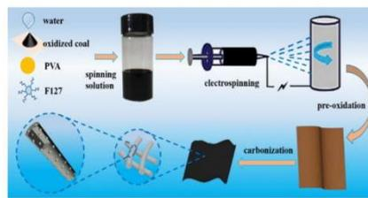
Fig. 1. The synthetic scheme of HPCNFs.
